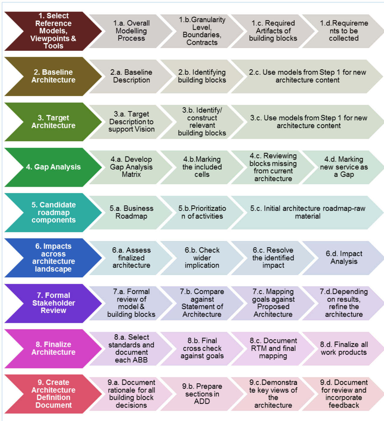
FIGURE 17: STEPS FOR PHASES OF ARCHITECTURE DEVELOPMENT METHOD
